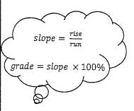
Ramps have a different code. They should have a slope between 1:12 and 1:10. Assume that anything less than 1:12 is not considered a ramp. A slope of 1:8 for a ramp is too steep and is strictly prohibited.
