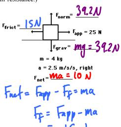
4. A 5-kg object is sliding to the right and encountering a friction force which slows it down. The coefficient of friction ("mu") between the object and the surface is 0.1. Determine the force of gravity, the normal force, the force of friction the net force, and the
