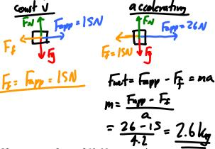
16. If you exert a force of 60. N on a car, it moves at a constant velocity. (i.e. there is a frictional force of 60. N) What is its mass if when you exert 80 N on it, it accelerates from rest to 2.0 m/s in 100.
